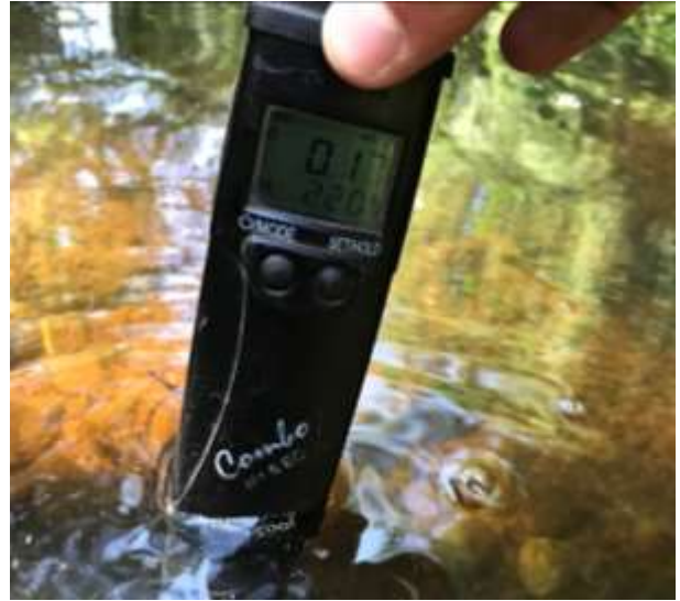
Figure 5.2. Water temperature reading taken to make sure that surveys are carried out in temperatures below the threshold for electric fishing to reduce stress to captured species.
